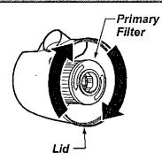
Before replacing the filter it is a good idea to clean the inside of the dust bin and lid area.
